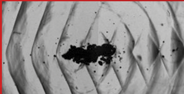
Shockwave formation in gel
