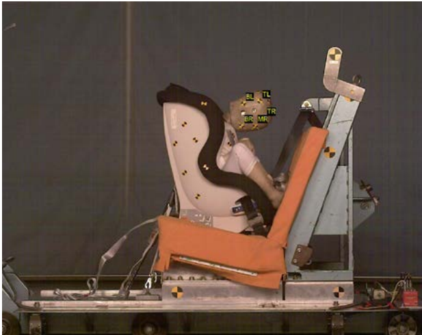
The orientation and 3D movement of the surveyed dummy head is measured by TEMA Pro 6DoF from a single camera view.
