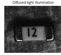
The entire contact is uniformly irradiated and its flat surface is not emphasized.
