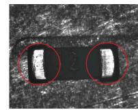
The contact's flat surface is emphasized by irradiating high-brightness light from the telecentric lens in the same axial direction as the camera.
